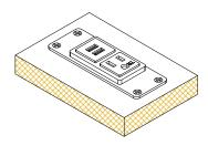
Step 3: a. Screw the four nuts onto each of the four studs below the mounting tabs and tighten.
