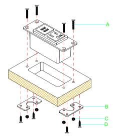
Step 2: Insert outlet from top and slip the mounting tabs over the threaded studs.
