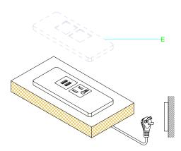
Step 4: Attach the cover; Connect to power supply.
