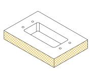
Step 1: Cut hole in wood for outlet.
